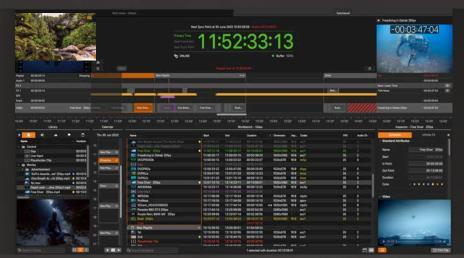
just play pro is an automated singlechannel, 24/7 master control playout solution supporting SD, HD, and UHD resolutions. It seamlessly delivers video playout over SDI or IP, integrating live feeds, triggered events, and realtime graphics ensuring reliable, uninterrupted broadcast playout operations.
